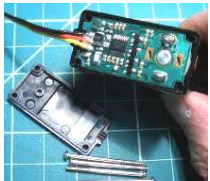
This photo shows the HS-311 servo with the back removed. The motor is on the right side of the housing
